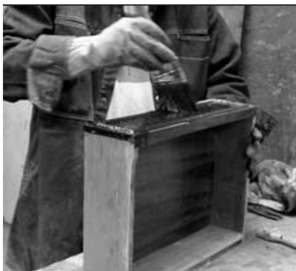
Brush paint stripper onto the furniture surface in one direction.
