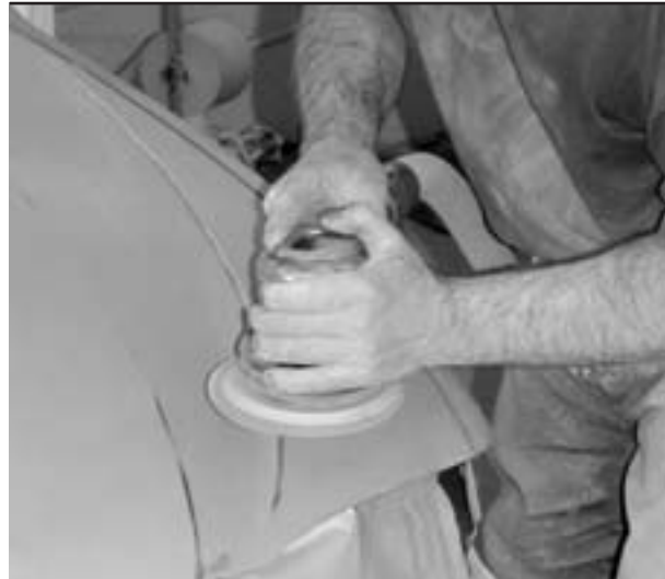
Sand the surface before applying paint stripper.
