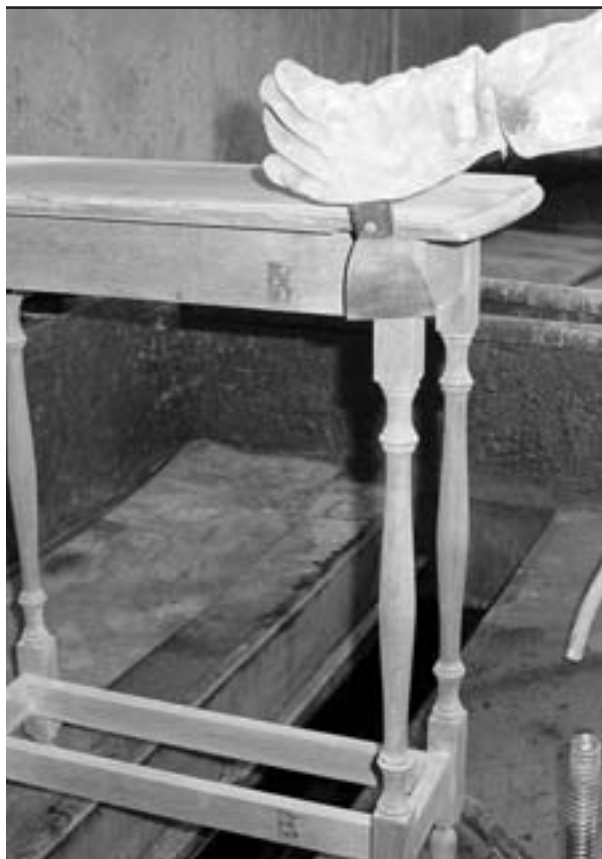
Begin scraping at the top of the furniture item and proceed downward.
