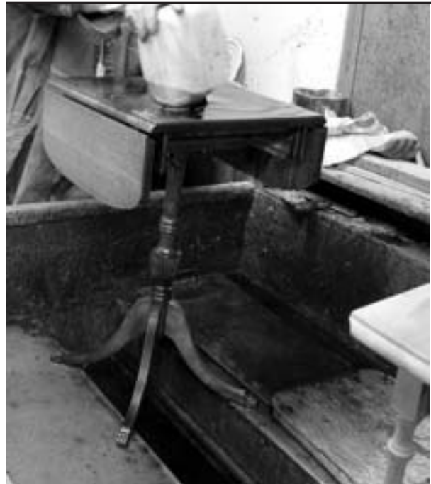
Place furniture item close to the flow-over tank drain to catch excess paint stripper.
